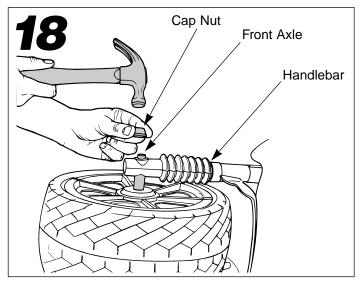
• Slide the front axle through the handlebar.
